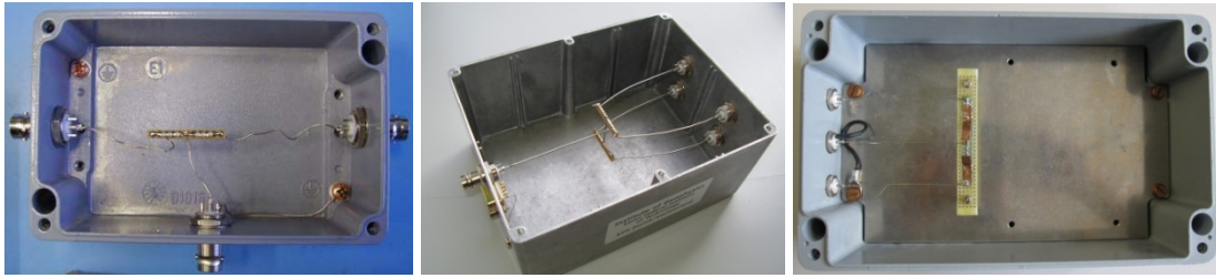
Figure 4-19 The line of successful TM simulator designs in a large box, all based on SMD capacitors. First simulator design (left), the dual 10 \mu\text{m} and 100 \mu\text{m} TM simulator (middle) and the latest design (right)
